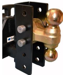
Dual Ball Installed in 210 Accessory Channel Hitch
