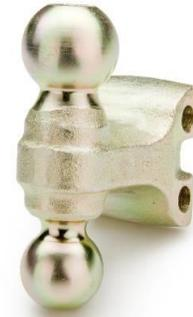
The towing capacities of the TeleSwivel 210 Accessory Channel are **7,000 lbs. gross trailer weight and 700 lbs. tongue weight** when towing with the 2 5/16" ball, and **5,000 lbs. gross trailer weight and 500 lbs. tongue weight** when towing with the 2" ball.
