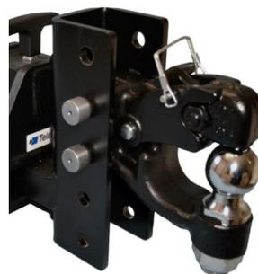
**Ball Pintle Installed in 210 Accessory Channel Hitch**
